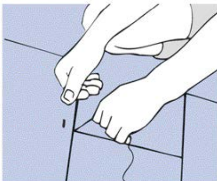
INSERTING REPLACEMENT SLATE
